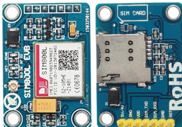
Figura 9: SIM800L EVB Modem
