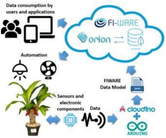
Figure 1: Rachel IoT smart plant architecture
